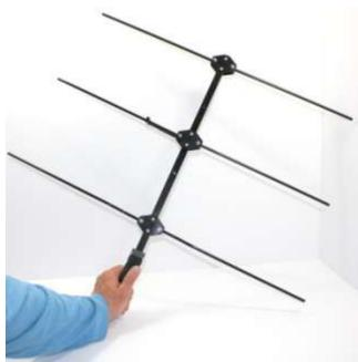
Figure 1 A three element Yagi antenna
