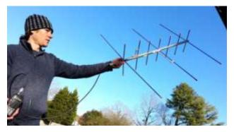
will need either a dual band colinear Figure 3 A dual band Yagi for use with satellites or dual band Yagi antenna. The latter, seen in the picture here Error! Reference source not found., can be pointed by hand at the predicted position in the sky, but it is the most "poke you in the eye" prone antenna ever designed!
